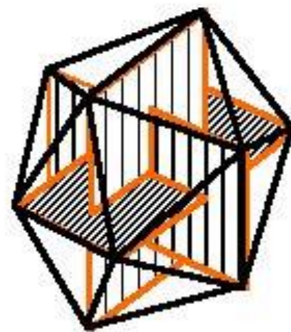
Linking the corners of rectangular planes builds an icosahedron
